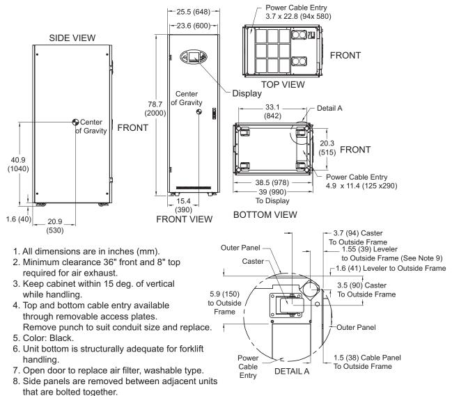
9. Leveling feet are not designed to carry the full weight of the cabinet. Finger-tighten leveler against the floor, then tighten with a wrench less than two turns for friction fit against floor.
